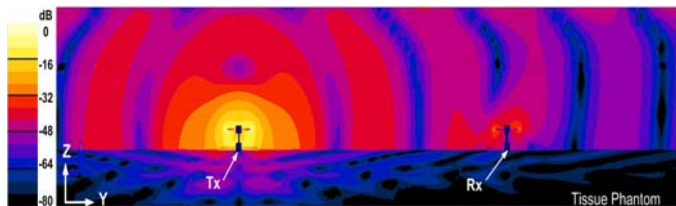
Fig. 8. HM-MPA antenna coupling simulation results showing normalised E-field magnitude through TX feedpoint.
