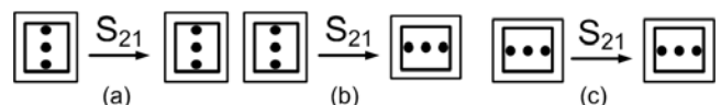
Fig. 10. HM-MPA orientation for S_{21} coupling measurements (a) Broadside, (b) Orthogonal and (c) End-fire.
