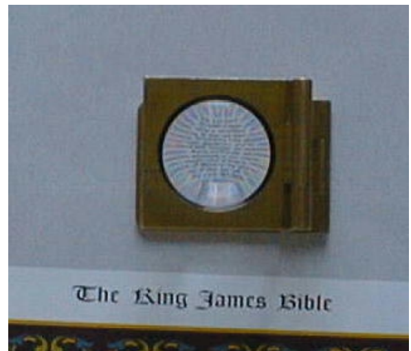
Fig. A complete bible printed on one poster. Standard offset printing with distinct letters made of "track-width" 25 um.
