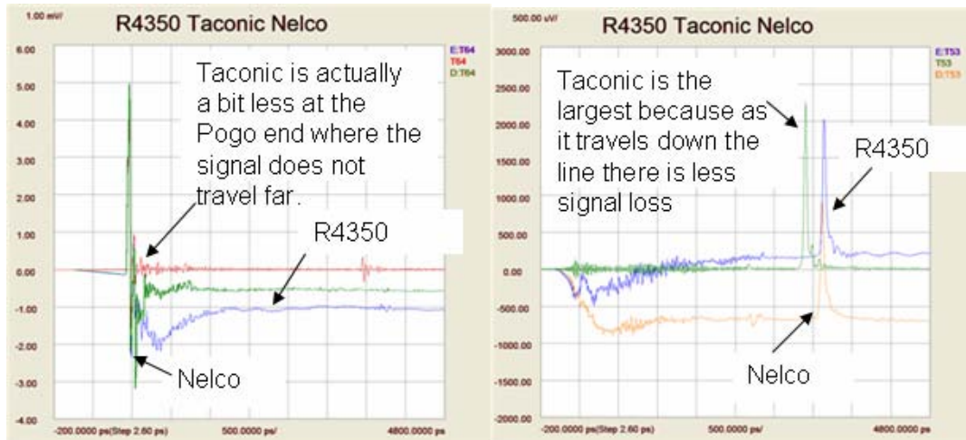
Figure 19: FEXT at the SMA end (left) and NEXT at the Pogo Block (right).
